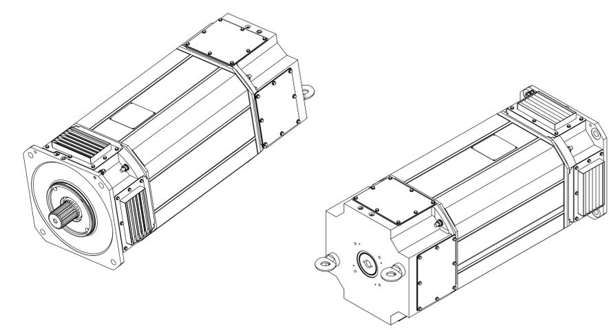
TYPICAL POSITION FOR EARTH STUD 1/2" UNC MINIMUM SECURED BY LOCKNUT (EARTH STUD AND FITTINGS ARE ZINC PLATED). EARTH STUD TO BE A CLEAN CONNECTION FITTED PRIOR TO PAINTING.
